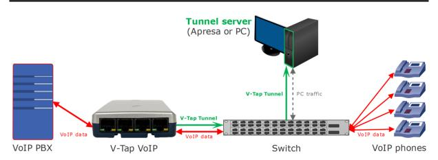
A connection between V-Tap and PC software (or Apresa) is needed to get the recorded data automatically into a user accessible database. The following checklist can be used to setup this Tunnel connection:
